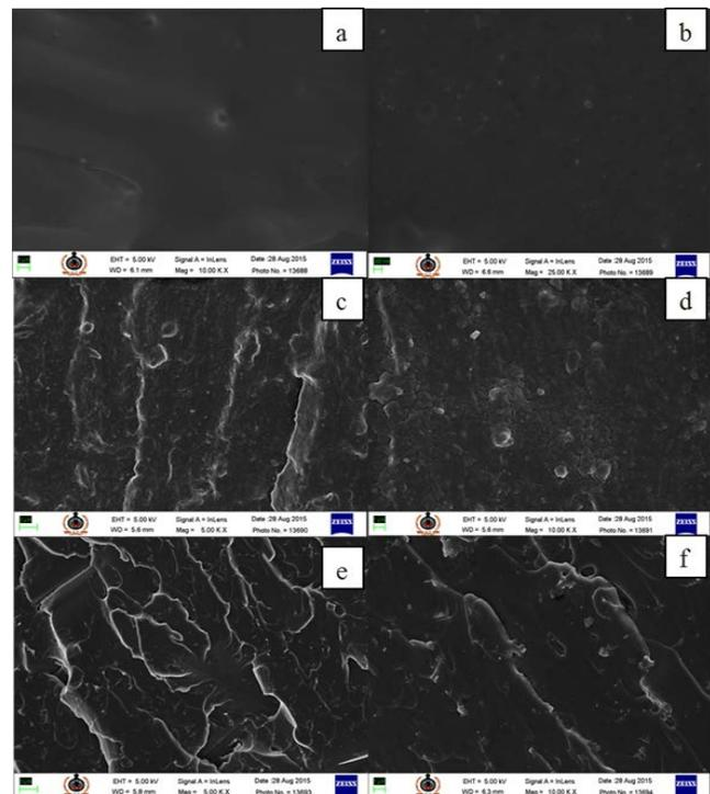
Fig. 3: SEM images of epoxy composite: Pristine epoxy (a & b), fractured epoxy composite with 0.5% carbon non solvent method (c & d), solvent method (e & f)
