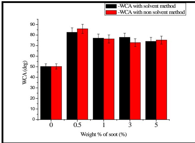
Fig. 4: Weight % of camphor soot in epoxy matrix v/s water contact angle
