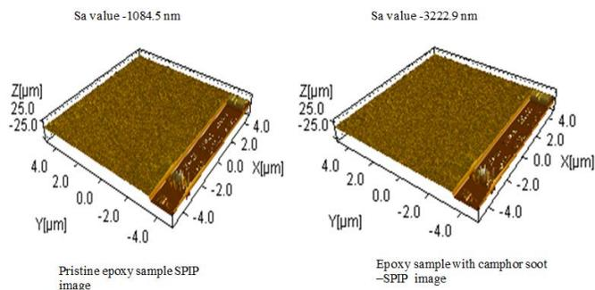
**Fig. 5: SPIP image of the clear epoxy and epoxy composite with Sa value**
